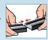
**Hint:** If necessary excess product can be cured by activator Loctite® 7455. Spray or drop activator onto excess product (not necessary with Loctite® 3090).
